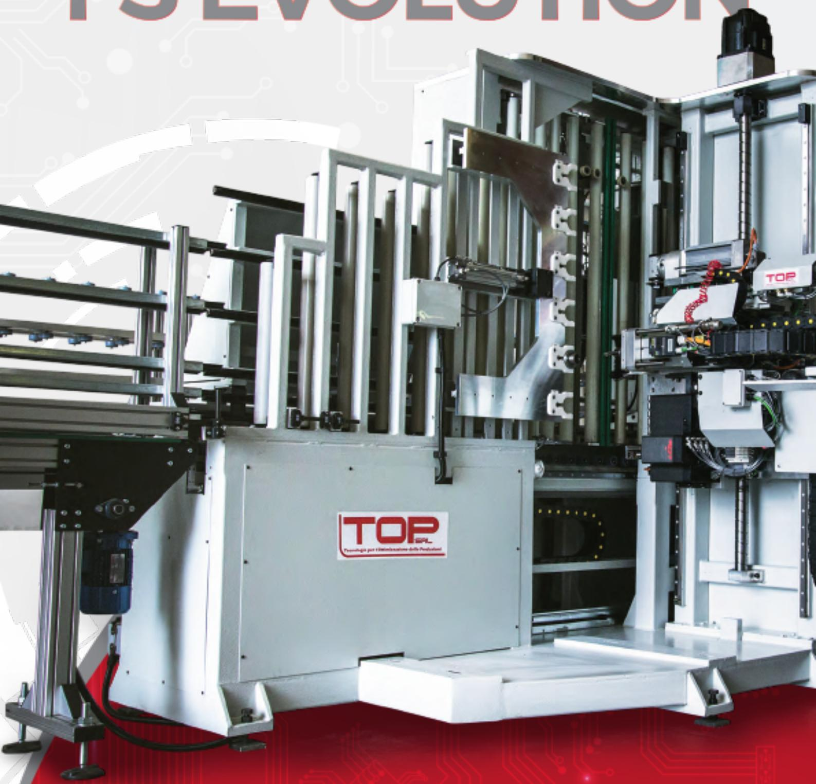
**FS-EVOLUTION - MACCHINA A CNC PER LA FORATURA, LA FRESATURA
